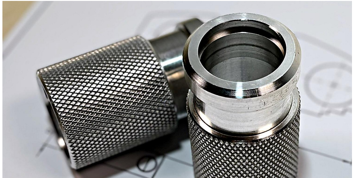
KNURLED BUSHINGS – THREAD, UNDERCUTS, CYLINDRICAL SURFACES.
